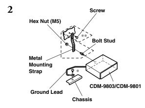
Reinforce the head unit with the metal mounting strap (not supplied). Secure the ground lead of the unit to a clean metal spot using a screw (\*) already attached to the vehicle's chassis.
